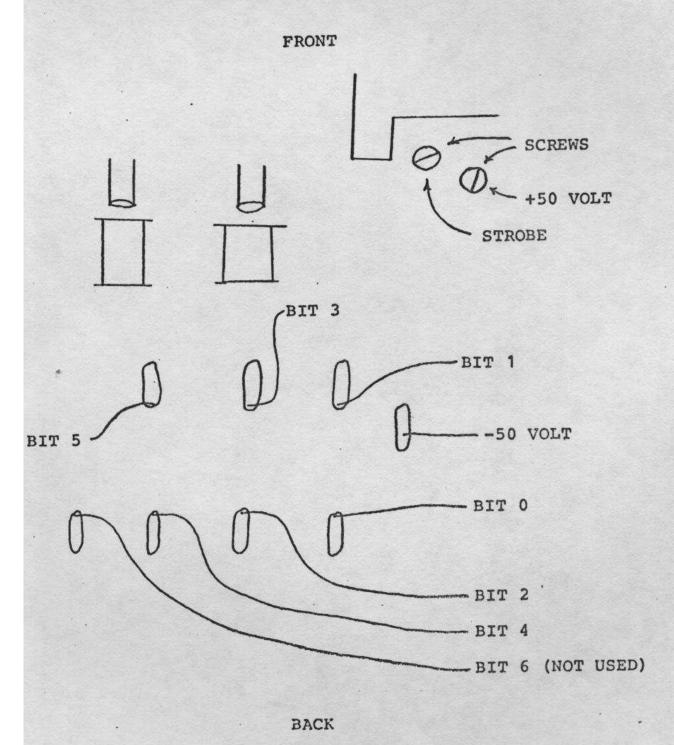
WIRES ARE SOLDERED TO THE UNDERSIDE OR TOPSIDE OF THE BIT SWITCHES
