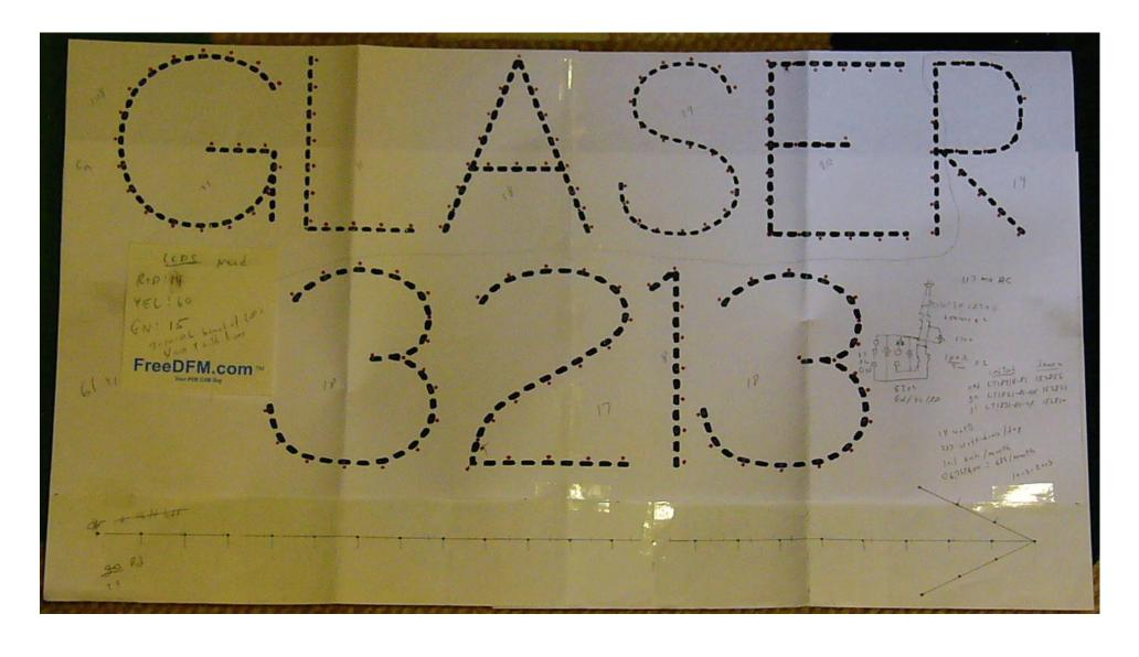
Trace font for kids (TRACFK\_\_.TTF) used to make a sign in PrintShop as a stencil Front and back are 19 inch rack panels. Holes drilled and LED's super-glued in place. Attached together about an inch apart with 10-32 machine screws/nuts.
